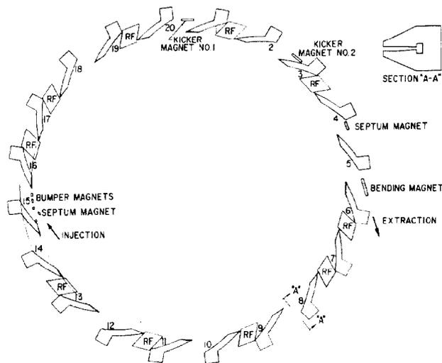
Fig. 1. Schematic View of the 1500-MeV FFAG.
