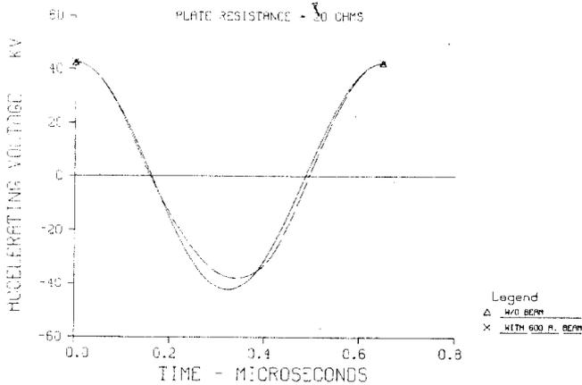
Fig. 3(a). Gap voltage waveforms with full loading and no loading with an amplifier impedance of 20 ohms.
