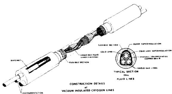
Fig.5 Typical construction of the cryogen transfer lines.
