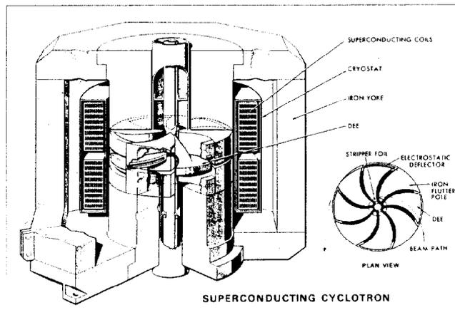
Fig. 2 The Chalk River superconducting cyclotron diagrammatic.
