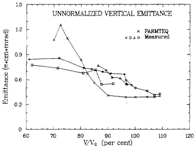
Fig. 7. Measured and predicted laboratory emittance areas as functions of RFQ vane voltage (vertical plane).
