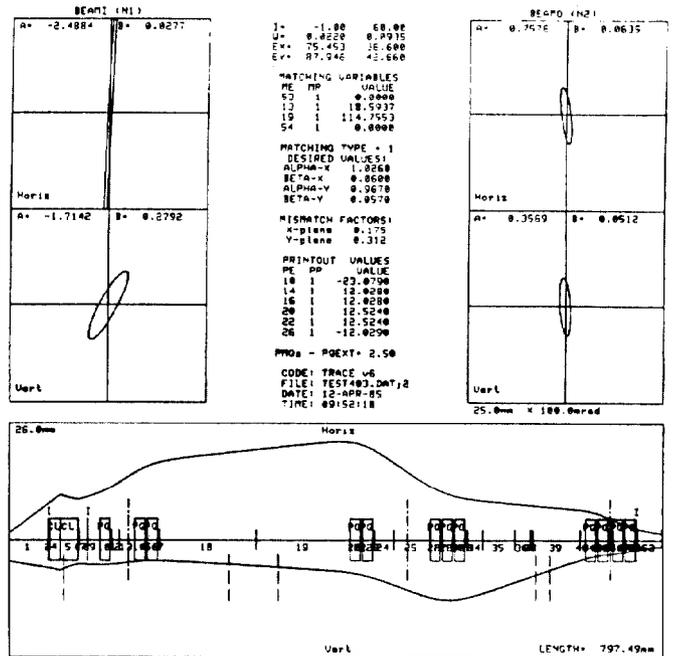
Fig. 2. TRACE beam-transport calculation showing mismatch of beam input to RFQ.
