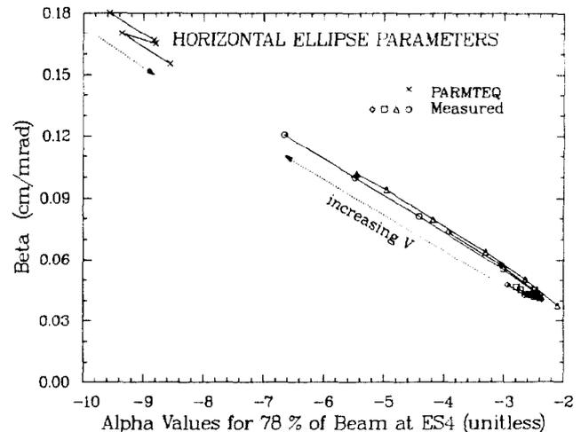
Fig. 4. Locus of ellipse parameters  $\alpha_x$  and  $\beta_x$  as RFQ vane voltage is varied. Both measured and calculated values are shown.
