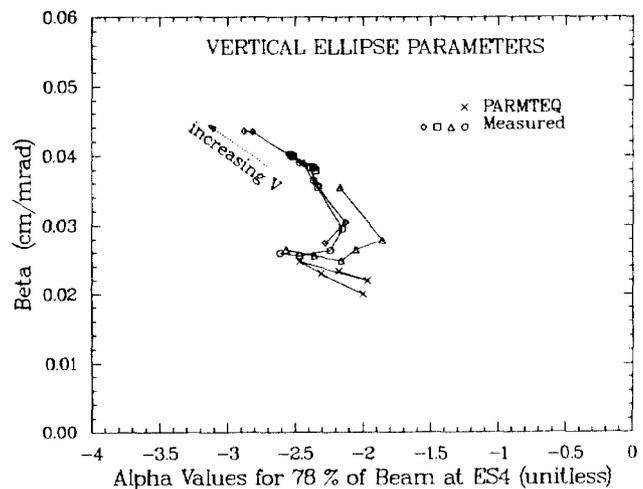
Fig. 5. Locus of ellipse parameters  $\alpha_x$  and  $\beta_x$  as RFQ vane voltage is varied. Both measured and calculated values are shown.
