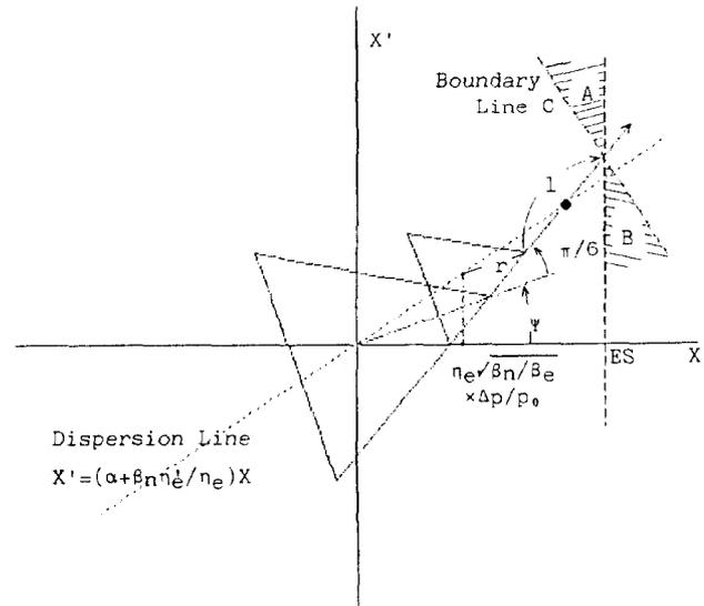
Fig. 2 Overlap of outgoing trajectories on the normalized phase space at ES
