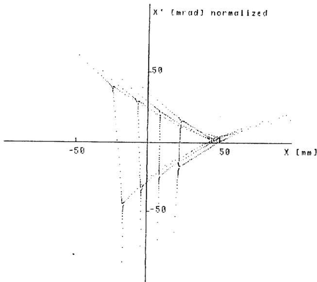
Fig. 3 The separatrices and outgoing trajectories of beams with  $\Delta p/p_0 = 0.0, 0.2, 0.4$  and  $0.6\%$ , respectively, at ES ( $\alpha=0$ )
