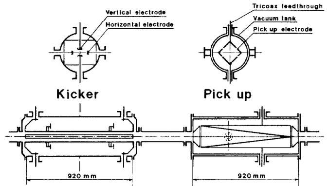
Fig. 1 : Kicker and pick up as installed in the PS ring
