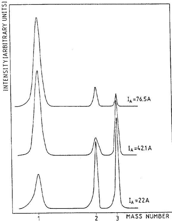
Fig. 4 Mass spectra of the extracted beam at  $I_A = 22A, 42A$  and  $76A$  showing relative contributions of  $H_1^+, H_2^+$  and  $H_3^+$  at  $U_A = 90V$ .
