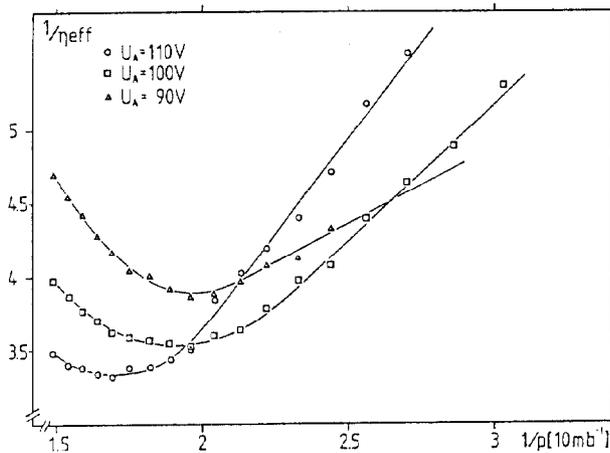
Fig. 2 Reciprocal effective ionisation efficiency  $1/\eta_{eff} = I_e/I_i$  as function of reciprocal source pressure  $1/p$ .
