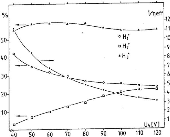
Fig.5  $H_1^+, H_2^+$  and  $H_3^+$  contents in the extracted beam as function of arc voltage  $U_A$  at arc current  $I_A = 22A$ . Dots represent inverse ionisation efficiency  $1/\eta_{eff}$  as function of  $U_A$ .
