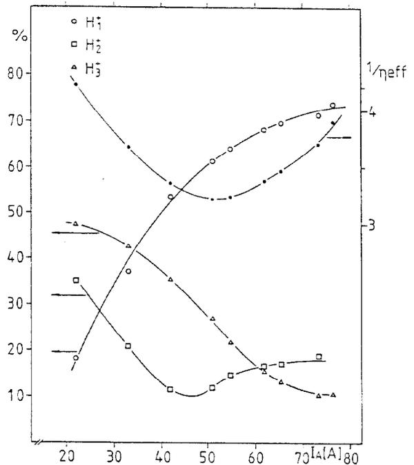
Fig. 3  $H_1^+$ ,  $H_2^+$  and  $H_3^+$  contents in the extracted beam as function of arc current  $I_A$  at arc voltage  $U_A = 90 \text{ V}$ . Dots represent inverse ionisation efficiency  $1/\eta_{eff}$  as function of  $U_A$ .
