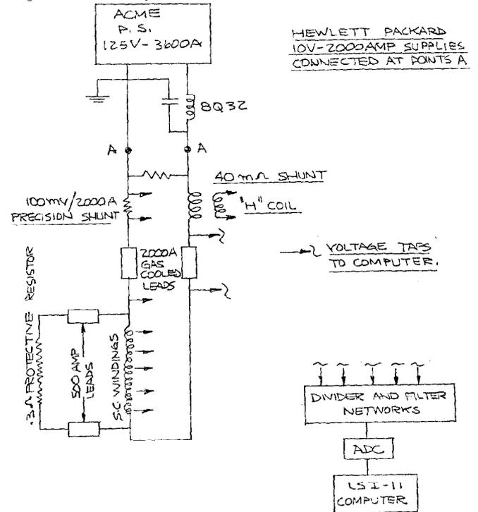
Fig. 1. Schematic showing the arrangement of the power supply and the instrumentation connections for the "D" bend dipole tests.
