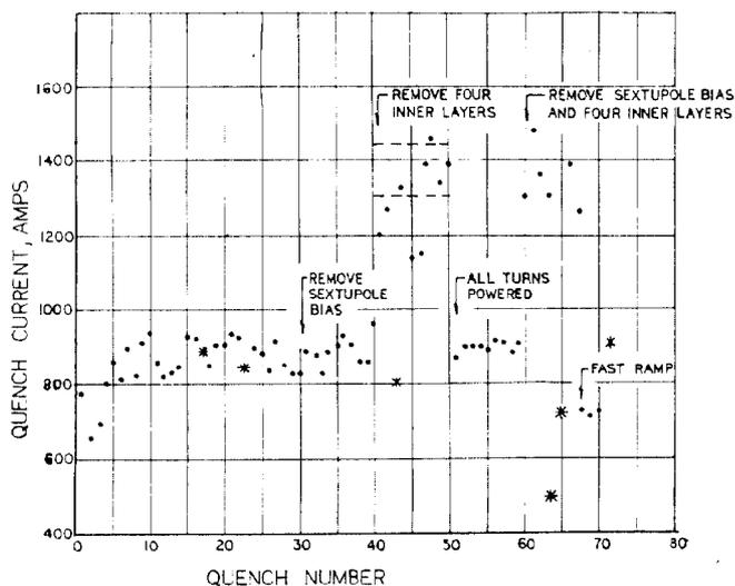
Fig. 2. Quench current versus quench number for the "D" bend dipole magnet.
