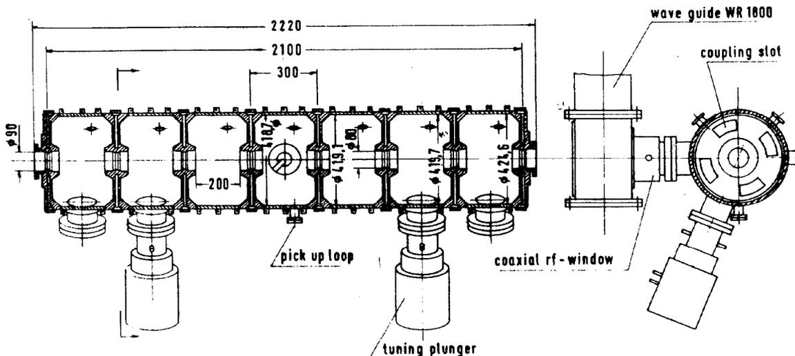
Fig. 1: PETRA new type 7-cell acceleration cavity (500 MHz)
