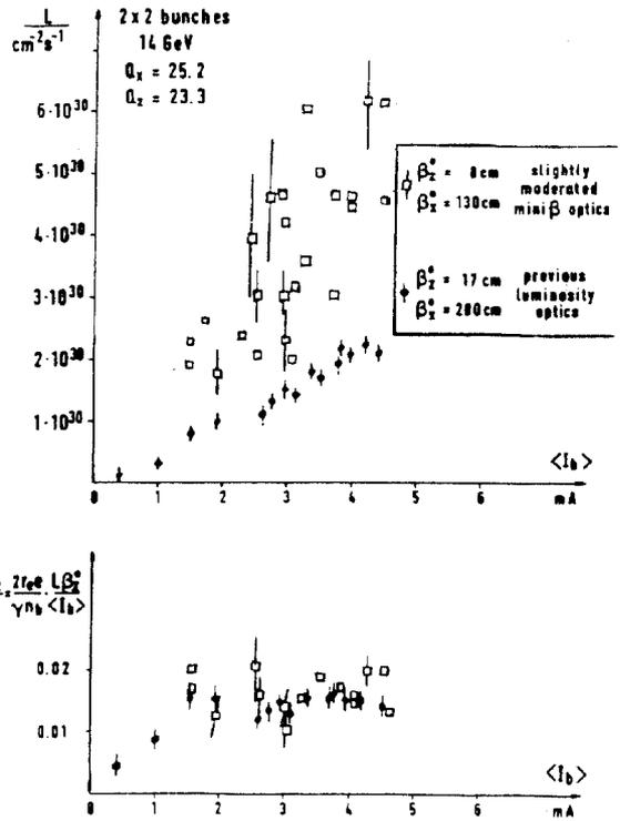
Fig. 4: Comparison of measured luminosity and vertical linear tune shift at 14 GeV with 2x2 bunches as a function of bunch current  $I_b$
