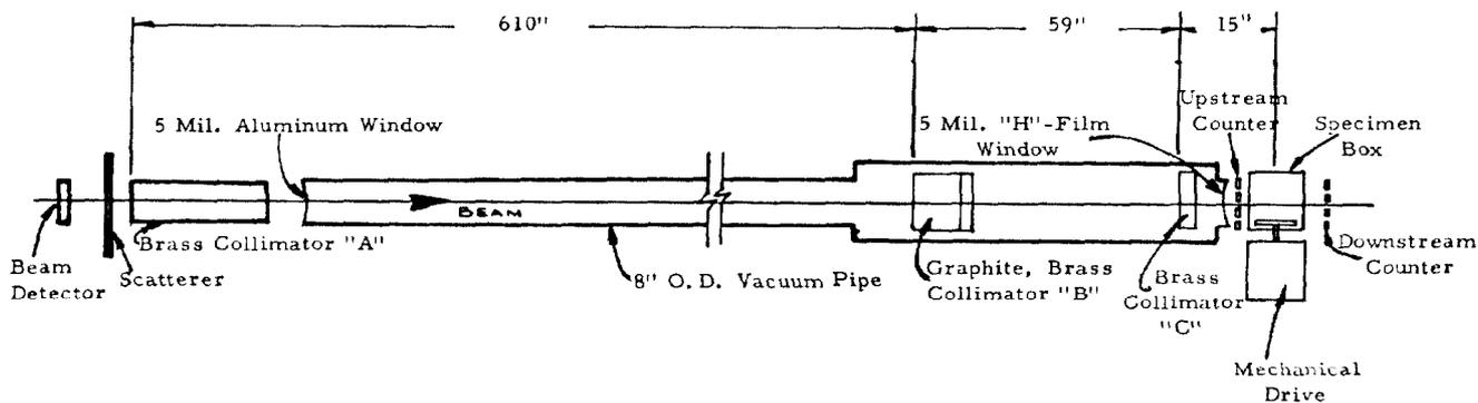
Figure 2 - Proton Radiography Beam
