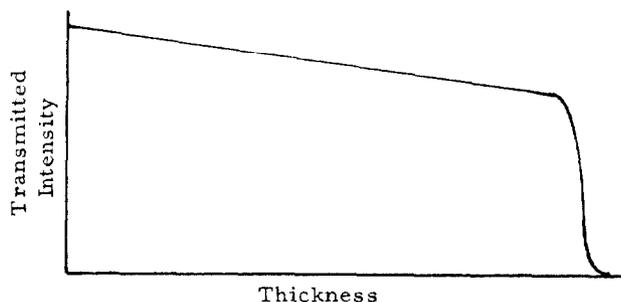
Figure 1 - Proton Range Curve
