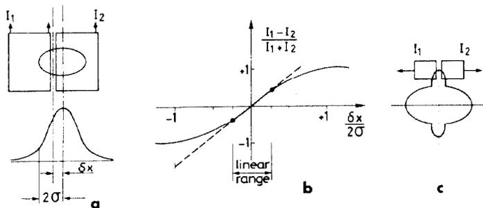
Fig. 3 : Spectrometry: a) principle of measurement with a split-plate detector; b) response of a split-plate for a Gaussian distribution; c) beam cross section in the image plane.
