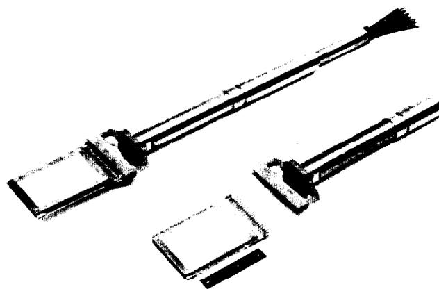
Fig. 4 : SEM-grid detectors: they are fixed on the plunging arm by mean of a plug-in socket
