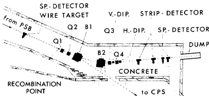
Fig. 1 : Layout of measurement line.
