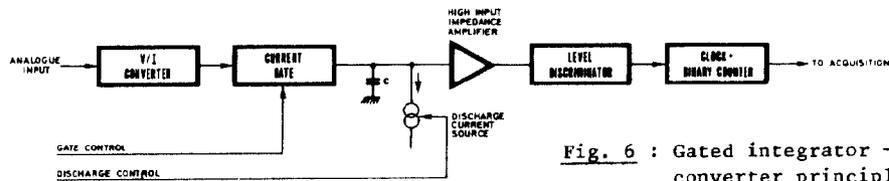
Fig. 6 : Gated integrator - converter principle.
