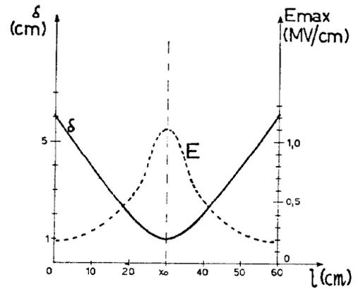
Fig.5 - Ring spread and maximum field versus drift length.
