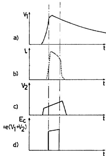
Fig.4 - Current and voltage patterns - a)diode voltage; b)current after energy selector; c)linear induction accelerator voltage; d)beam energy.
