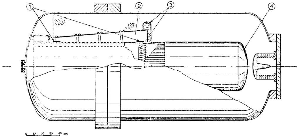
Fig.2 - Tesla transformer - 1)Secondary windings; 2)primary windings; 3)guard rings 4)HV terminal.
