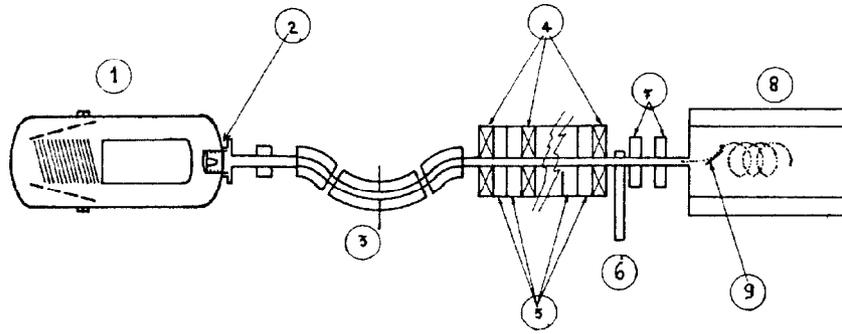
Fig.3 - Complete system - 1)Tesla transformer; 2)diode; 3)energy selector; 4)focusing coils; 5)linear induction modules; 6) beam monitor; 7)focusing and matching quadrupoles;8)ANEL 1 magnet; 9)injection septum.
