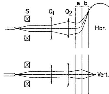
Fig.1 - Injector optics - S) Solenoid; Q<sub>1</sub>, Q<sub>2</sub>) quadrupoles; a) region of overcompensated field; b) region of compensated field.
