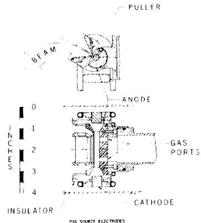
Fig. 2. Cross-sections of anode-puller region.
