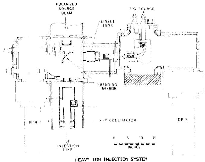
Fig. 1. PIG source injection system showing source, focusing lens, bending mirror, Faraday cups, and scanning wires for beam monitoring.
