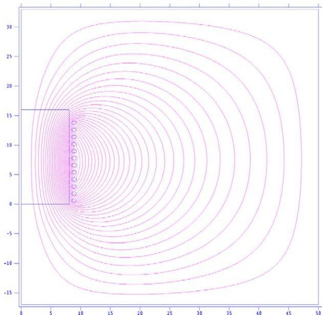
Figure 4: Superfish simulation of the 12-turn inductor.
