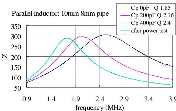
Figure 3: Cavity impedance with 10-turn inductor.
