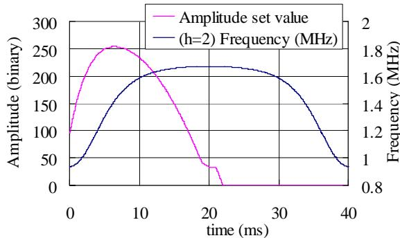
Figure 7: Amplitude and frequency for 25Hz operation
