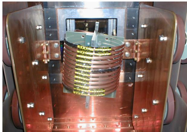
Figure 5: Air-cooled parallel inductor with thermo-labels.
