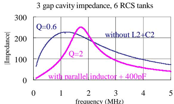
Figure 2: Cavity impedance with and without  $L_2+C_2$ .
