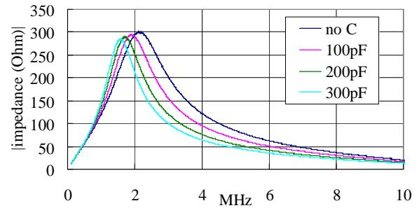
Figure 9: Cavity impedance with 14-turn inductor as function of parallel vacuum capacitor.
