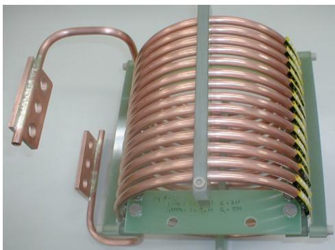
Figure 8: 14-turn inductor production version
