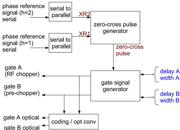
Figure 4: Block diagram of the CMT module, the chopper timing part.
