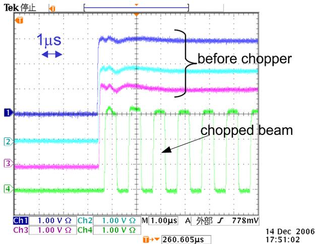
Figure 2: Chopped beam signals measured by current transformers.
