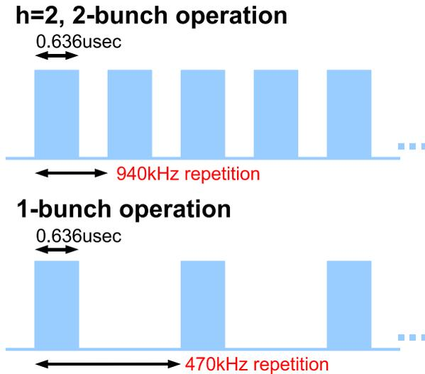
Figure 3: Intermediate pulses for 2-bunch and 1-bunch operation.
