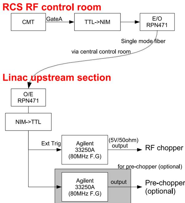
Figure 5: Signal transmission option with a function generator.
