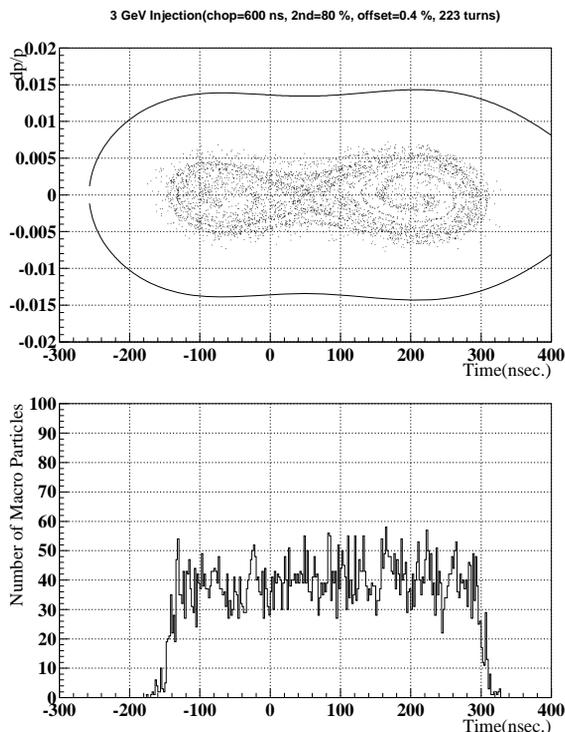
Figure 1: A typical bunch shape after injection using the multi-turn momentum-offset injection scheme. The second harmonic RF is also applied.
