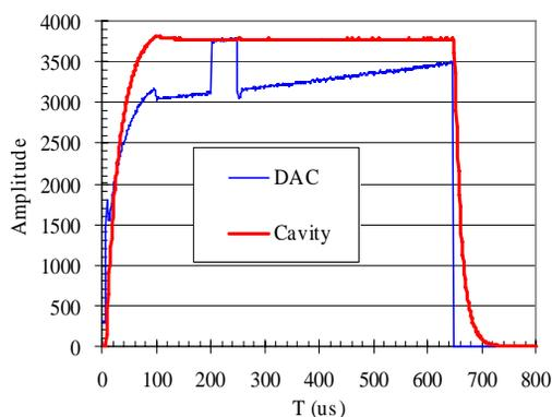
Figure 6: Amplitudes of the cavity and DAC outputs at SDTL3 with beam feedforward compensation.
