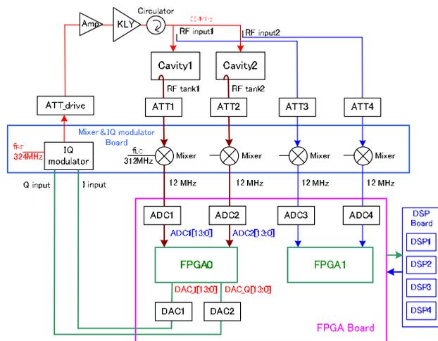
Figure 1: Block diagram of the RF feedback control system.
