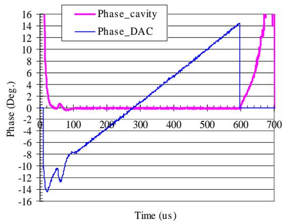
Figure 5: Phase of the cavity and DAC outputs at SDTL7.
