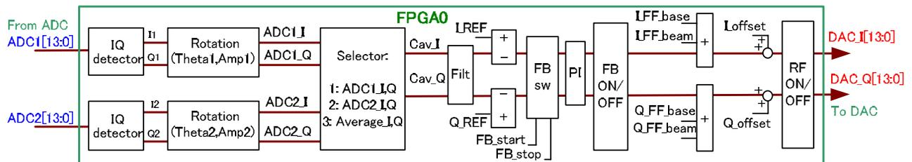
Figure 2: Block diagram of the digital feedback control in FPGA0.
