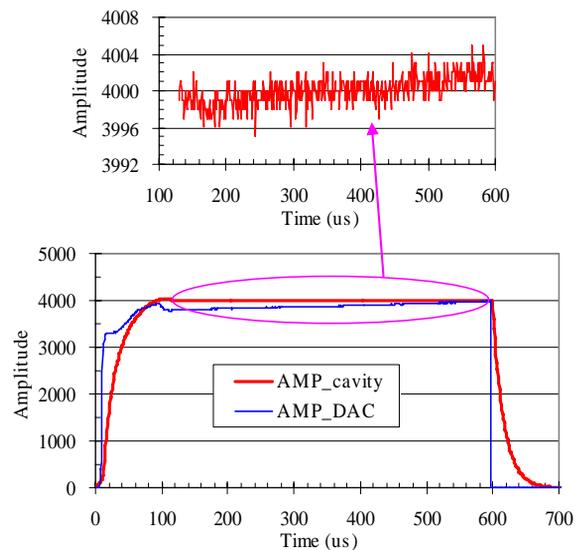
Figure 4: Amplitudes of the cavity and DAC output at SDTL7.
