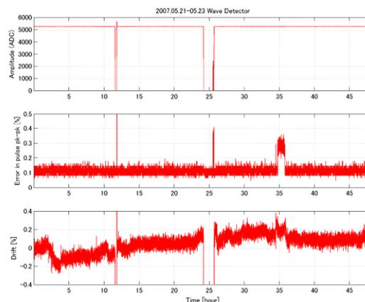
Figure 7: Stability of the RF feedback control system at DTL3.
