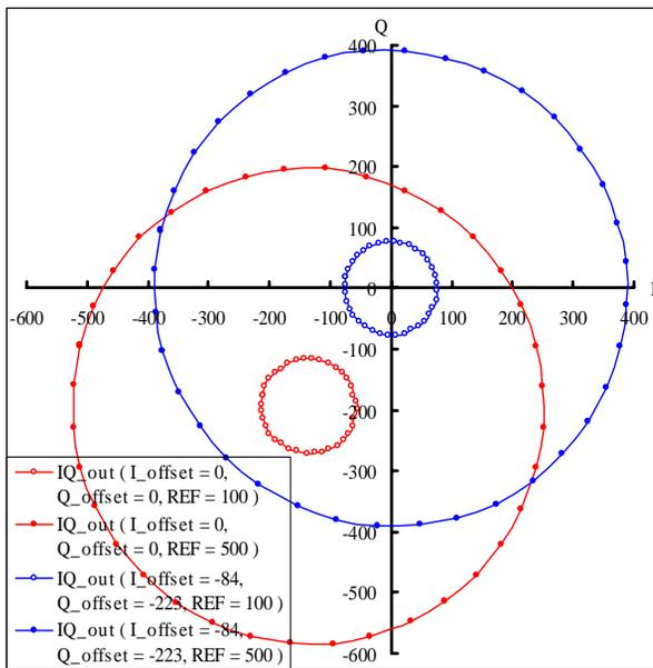
Figure 3: IQ modulator outputs at SDTL13 with or without IQ offsetting.
