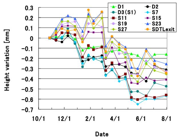
Figure 4: Elevation of vertical markers measured since Oct. 2005. Horizontal axis is the measured date and vertical axis is the height change from Oct. 2005.
