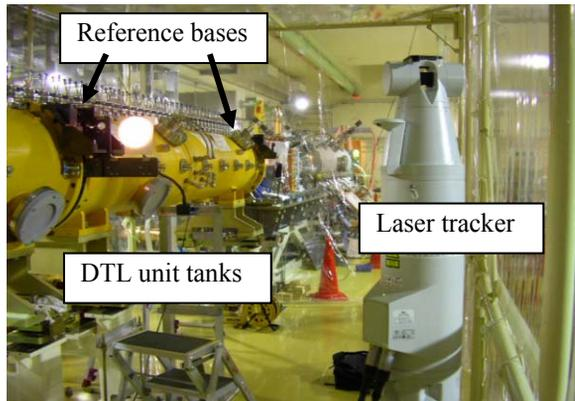
Figure 2: Laser tracker and reference bases on unit tanks.
