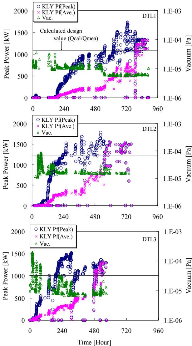
Figure 2: Conditioning histories of the DTLs. The scale of the averaging power is 1.625% (DTL1 & 3), and 1.5% (DTL2) of the peak power level.
