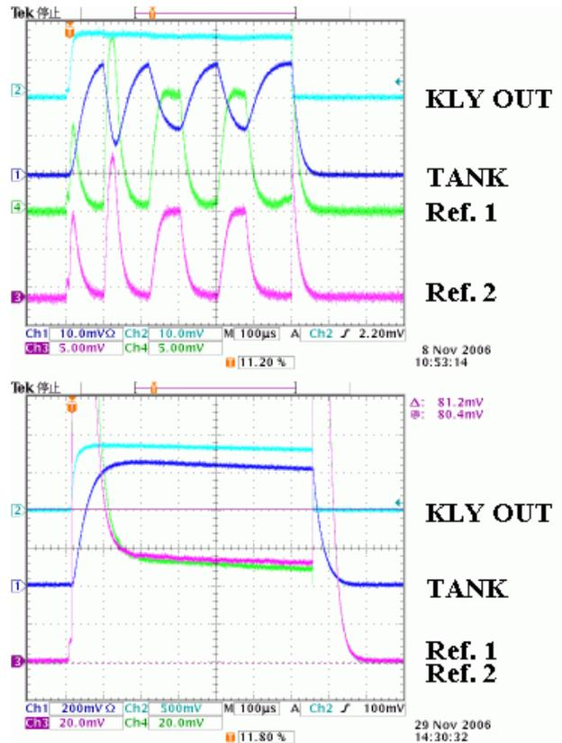
Figure 3: Waveforms of rf power for the DTL3. The topside picture is at the beginning of the conditioning (klystron output is 4kW) and the downside picture is at the end of the conditioning (Klystron output is 1.1MW). Note that the vertical scales are different.
