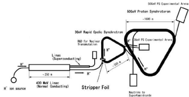
Figure.1 Schematic layout of the accelerator complex of J-PARC
