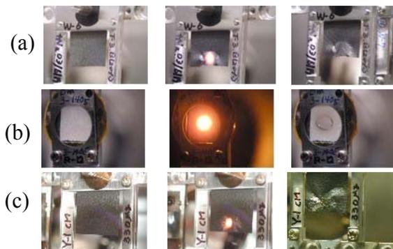
Figure.6 Photographs of (a) a double-layered HBC-foil, (b) a DM-foil and (c) a CM-foil at different stages of irradiation.
