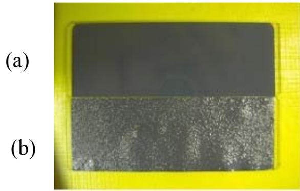
Figure.4 Photographs of carbon layers on slide glasses. Represent an HBC-foil of  $370 \mu\text{g}/\text{cm}^2$  and is for a Cluster-foil of  $140 \mu\text{g}/\text{cm}^2$  made by the CADAD method.
