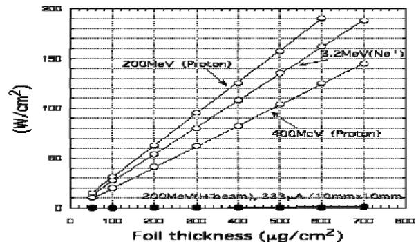
Figure.2 Energy deposition as a function of foil thickness for 200 MeV, 400 MeV and  $\text{Ne}^+$  DC beam.
