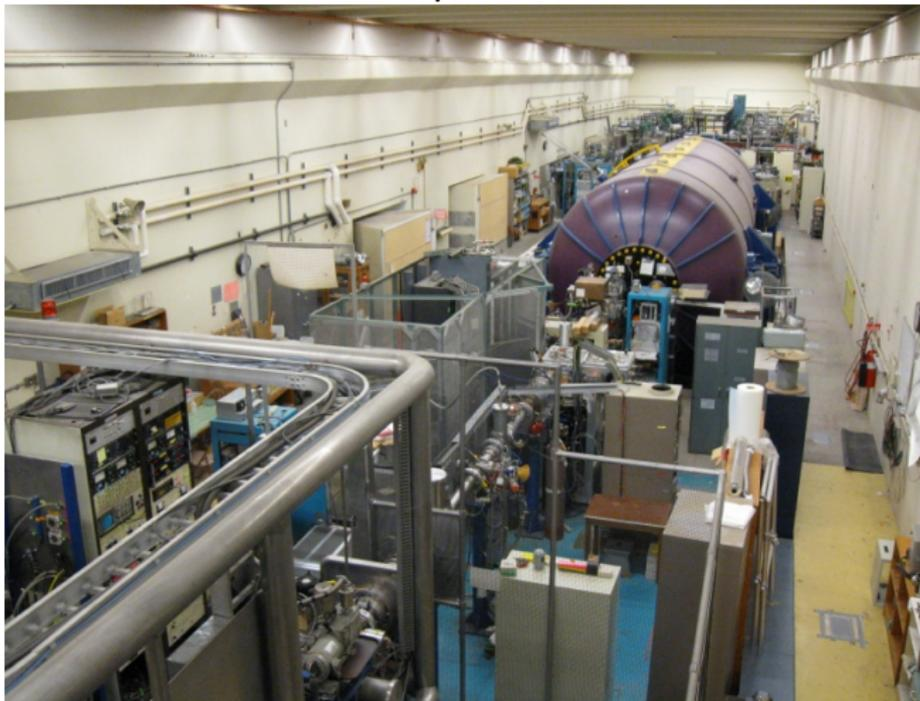
Model FN tandem VDG, pelletron charging
