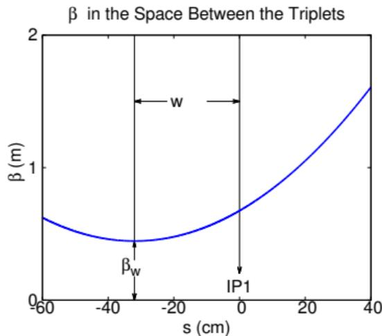
$\beta_{w_r}$  and  $w_r$  are measured in the LHC using the  $k$ -modulation technique<sup>3</sup>.
