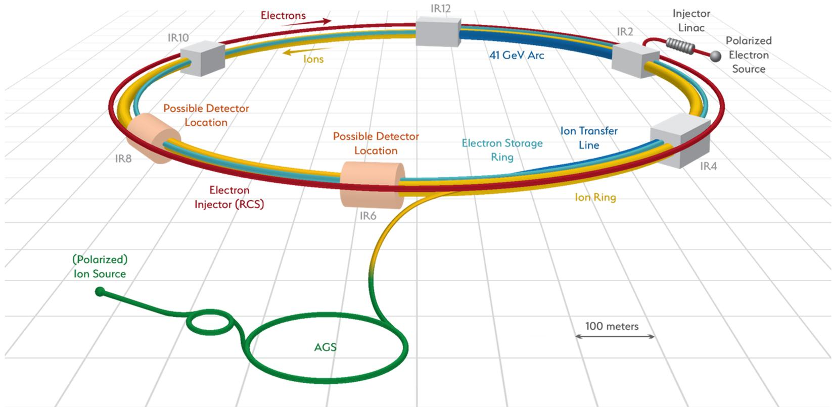
Electron complex to be installed in existing RHIC tunnel – cost effective
