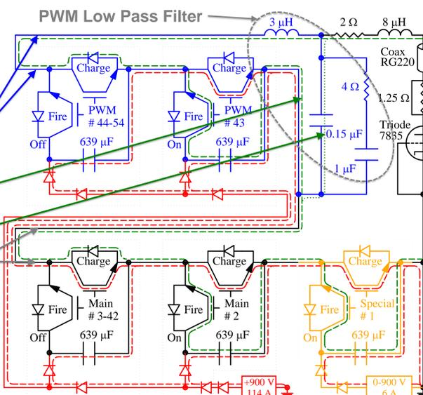
Simplified 5 Cell Marx Modulator Schematic (Charging Current Path in Red, Firing Path in Green)
