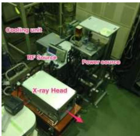
Figure 5: 3.95 MeV portable X-band linac based X-ray source. The system consists of four units: X-ray head, magnetron, power, and chiller units.
