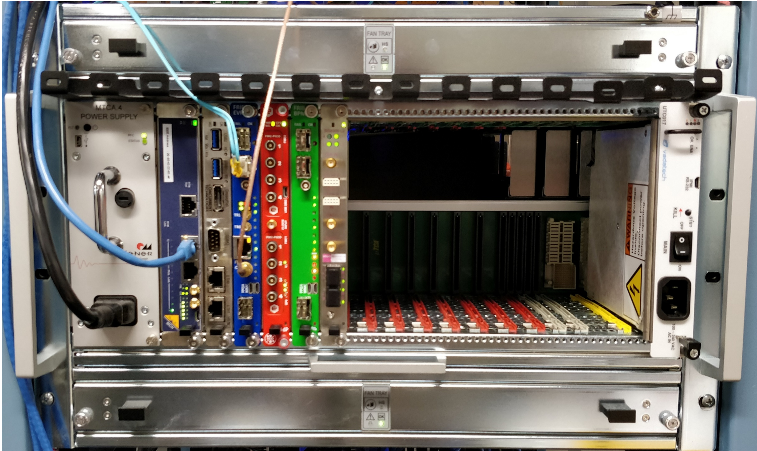
Figure 1: A \mu TCA crate with MCH, CPU, Event Receiver, Pico8, BPM and BCM cards.
