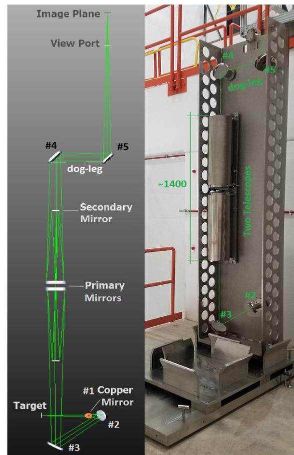
Fig. 5. Left side is the light pass in the relay lens. Right side is the target vessel mounting frame with prototype board with optical elements of relay lens. The detection module with cameras is not shown here.
