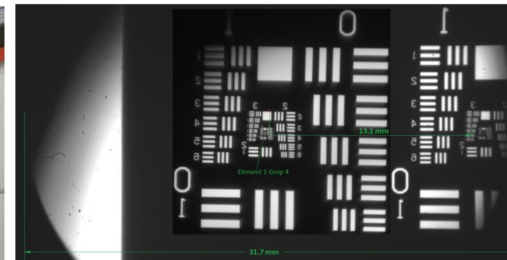
Fig. 7. Image of USAF-1951 on camera sensor after telecentric lens. Two images near center and edge of FOV are merged in one picture. Measured FOV is 31.7mm. Near center the element 1 in group 4 is still resolvable that corresponds to resolution 16 lp/mm. Resolution is reduced to 10 lp/mm at 13.1mm from the center.
