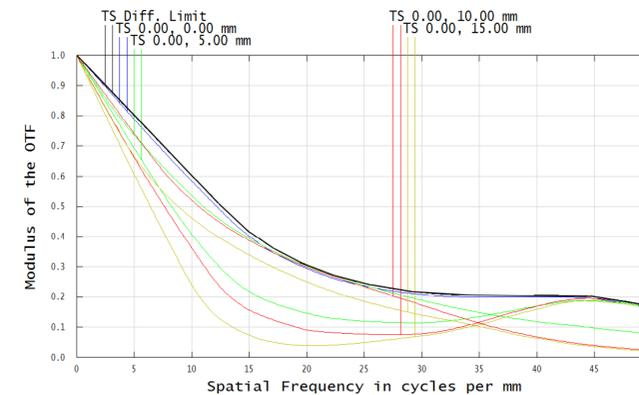
Fig. 4. Modulation Transfer Functions for axial point (blue) and for points at 5mm (green), 10mm (red) and 15mm (yellow) from axis. The black solid line describes contrast dependence for diffraction limited optical system.
