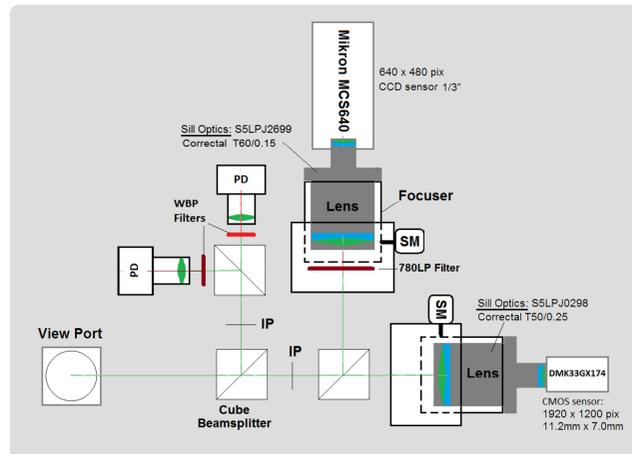
Fig. 2. Optical breadboard diagram. The cube beam splitters have 50% by 50% ratio. Here is IP – image plane; SM – stepper motor; PD – photodiode; WBP – wide bandpass filter. 780LP – longpass filter with cut wavelength 780 nm.
