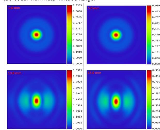
Fig. 3. Point Spread Functions for axial point and for points at 5mm, 10mm and 15mm from axis.
