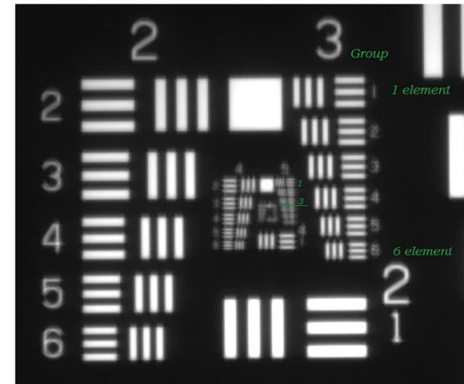
Fig. 6. Image of USAF-1951 in focal plane of the relay lens. Resolution is about 40 line pairs/mm and it is limited by astigmatic secondary mirror of second telescope. To obtain this image a camera with a 5.86 $\mu$ m square pixel was used.
