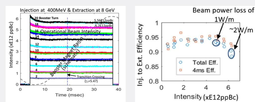
The Fermilab Booster suffers from injection losses at the few percent level, independent of beam intensity.
