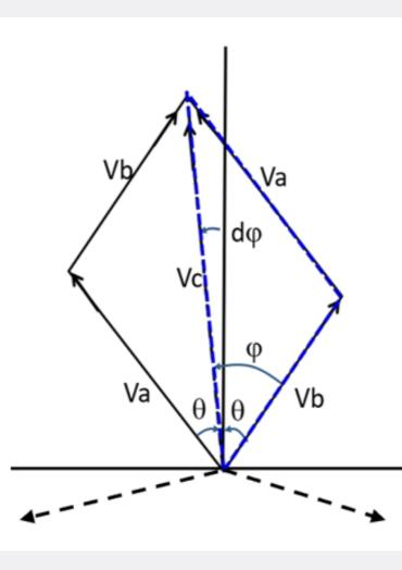
Adiabatic capture matches the debunched beam from the linac to the Booster RF buckets by gradually increasing the total Booster RF capture voltage. This is accomplished by dividing the Booster RF cavities A & B stations, which start out of phase and gradually phase in. Present operation finds best efficiency with a "neck" in which the total voltage decreases from a small value before it increases. We believe that neck may be covering for mismatched errors
