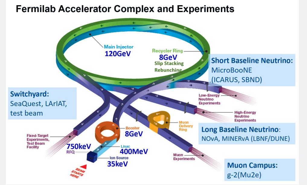
The Fermilab accelerator complex delivers high intensity hadron beams to a variety of HEP experiments.
