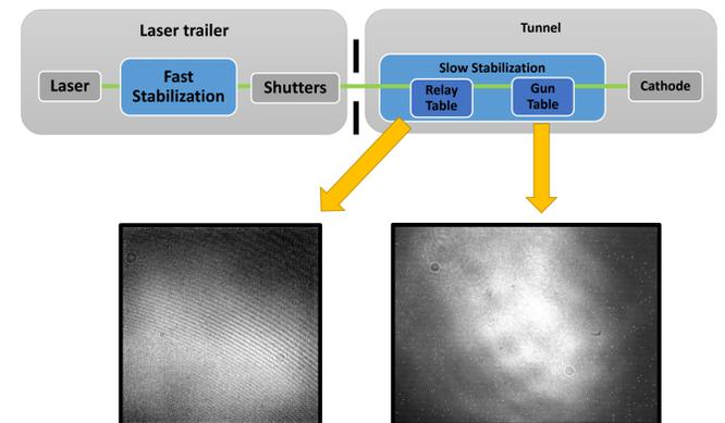
Example of laser beam profile on the relay table (left) and gun table (right) for the same beam through the transport in pulsed mode. The slow stabilization system was designed to handle both the relay table’s large, diffuse beam and the gun table’s highly structured beam with pulsed-to-CW dynamic range.
