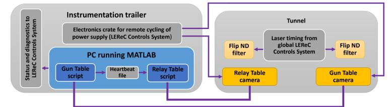
Conceptual layout of the slow stabilization system communication. Cameras are on a local network, with one-way communication to the network Controls System for diagnostics data.
