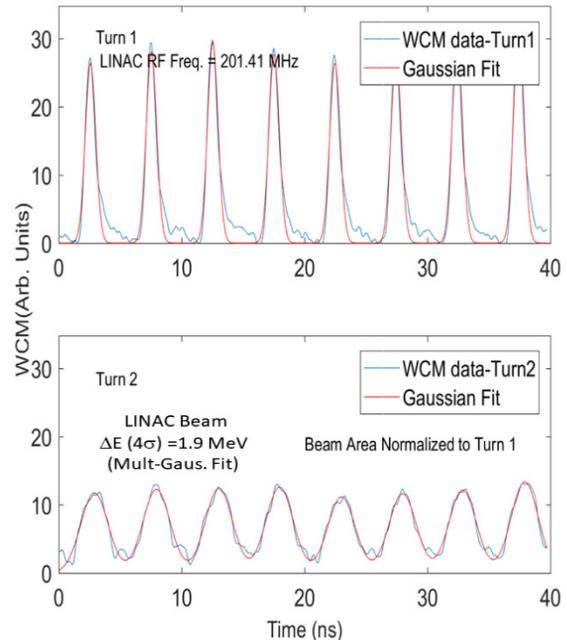
Figure 2: (a) Bunch profiles for 1<sup>st</sup> turn in the Booster and (b) multi-Gaussian fit for WCM data for the same beam on second turn. These arbitrarily chosen eight bunches with no overlapping bunches. Measured  $\Delta E$  are also shown.
