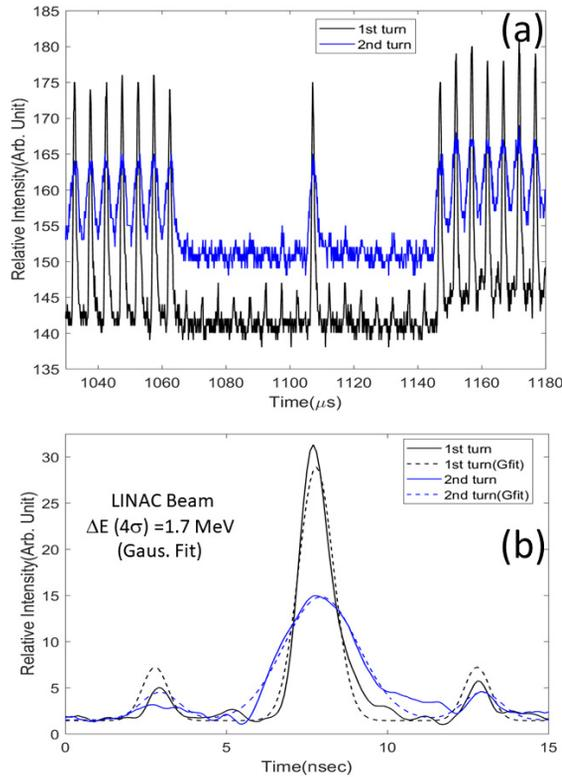
Figure 1: (a) Bunch profiles for 1<sup>st</sup> and 2<sup>nd</sup> turn in the Booster and (b) Gaussian fit to the untouched single bunch in the notch for 1<sup>st</sup> and 2<sup>nd</sup> turn. Measured  $\Delta E$  are also shown.
