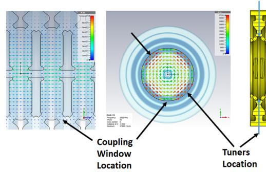
Figure 3: Tuners location with respect to coupling windows.
