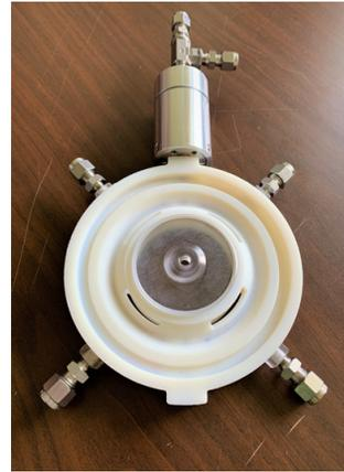
Figure 10: Photo of a 3D-printed single cell with one tuner assembly and inlets and outlets of cooling channels.
