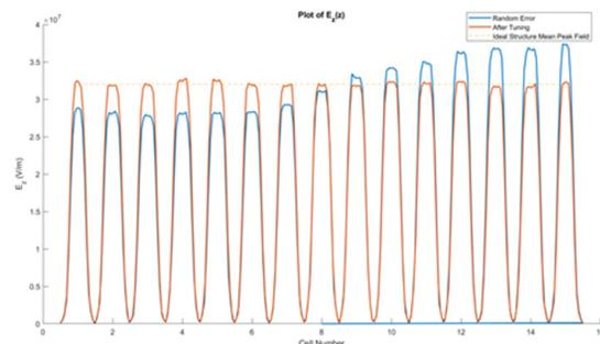
Figure 5: Longitudinal field profile (absolute value) along the structure including errors (blue) and after tuner adjustment for both frequency and flat field (red).
