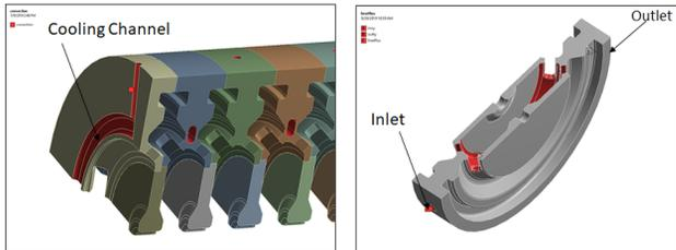
Figure 7: Cooling system design showing the cooling channels inlet and outlet.
