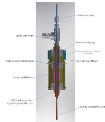
Figure 4: Tuner design and system assembly.
