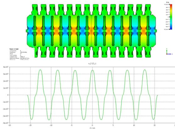
Figure 2: Electric field distribution in the 15-cell structure (top) and on-axis accelerating field profile (bottom).
