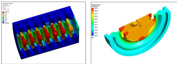
Figure 8: Temperature distribution assuming 4-bar pressure drop, the maximum temperature gradient is ~ 18 C.
