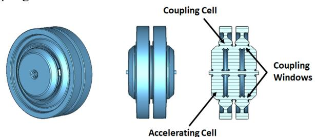
Figure 1: Geometry of an ACS structure with 3 accelerating cells and 2 coupling cells.
