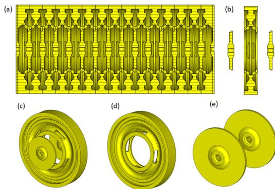
Figure 9: Fabrication procedure. (a) and (b) shows how the cavity is split into cells and disks. (c), (d) and (e) show how a single cell is built of a ring and two disks.
