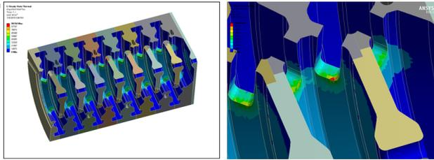
Figure 6: Loss distribution for 2.5 kW average power.
