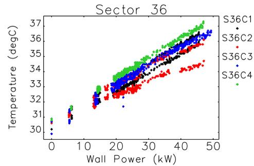
Figure 2: Temperature probe versus cavity wall power for sector 36 cavities. Two probes per cavity are shown. Data shows a linear dependence, which is not surprising.
