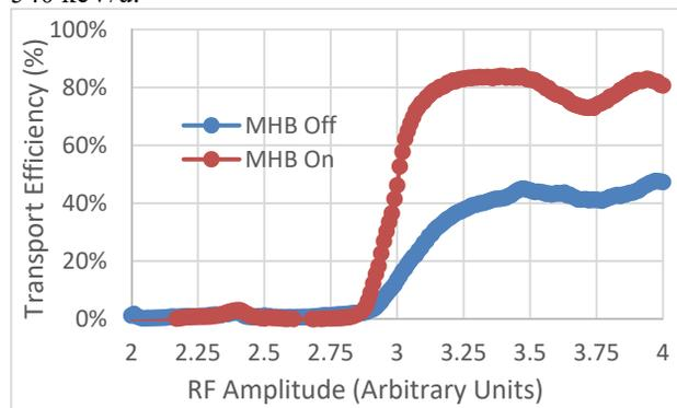
Figure 4: RFQ transport efficiency as a function of RF amplitude, with and without the multi-harmonic buncher.
