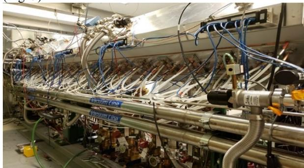
Figure 3: View of the back of the RFQ tank showing water cooling lines and return water temperature sensors.
