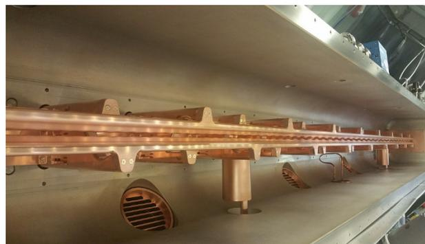
Figure 2: Copper components of the RFQ structure after installation.
