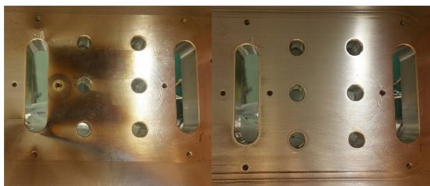
Figure 1: An area of the tank surface before and after the polishing procedure.
