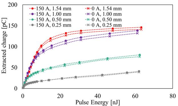
Figure 5: Extracted charge vs laser pulse energy variation with laser spot size for magnetized and non-magnetized beam (100 kV, 50 kHz, 70 ps (FWHM)).
