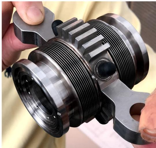
Figure 7: APS-U BPM with bellows prototype.
