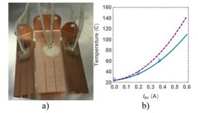
Figure 3: a) GLIDCOP RF fingers of the bellows with attached RTDs for internal temperature measurements. b) Internal temperature measurements at  $V_{RF} = 3MV$  (blue dots) and the data fit (dark cyan solid line). The dashed purple line is the predicted data at  $V_{RF} = 4.5MV$ .
