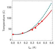
Figure 7: The internal temperature of the stripline electrodes vs. average current measured by the IR temperature detector (red dots). The red solid line is the data fit at  $V_{RF} = 3MV$ . The dashed dark cyan line is the predicted data at  $V_{RF} = 4.5MV$ .
