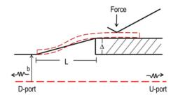
Figure 2: Simplified 2D model of the bellows.
