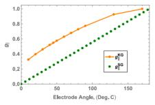
Figure 11: Longitudinal geometric factor as a function of electrode angle  $\phi$  for simplified geometry (SG) and for the stripline kicker geometry (KG).
