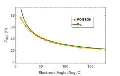
e 12: The longitudinal (orange) and transverse (green) acteristic impedances as a function of electrode angle lculated using the POISSON code for the stripline er geometry.
