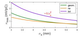
Figure 5: The loss factor as a function of bunch length for the bellows geometry.
