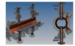
Figure 6: Diagnostic stripline with six IR view ports.
