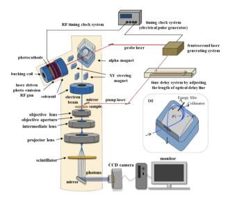
Figure 1: A schematic of the UEM with an alpha-magnet.
