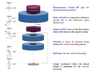
Figure 4: The design concept of bunch compression with a single-cell RF cavity.
