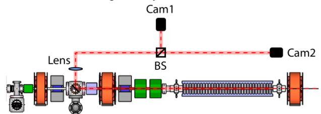
Figure 3: Alignment scheme for the e-beam and radiation in the PU; similar configuration is used for the KU.
