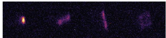
Figure 7: SR images of an individual electron undergoing large betatron oscillations in IOTA due to residual-gas scattering. (from left to right) fully damped single electron; large amplitude horizontal, vertical, and mixed betatron oscillations.
