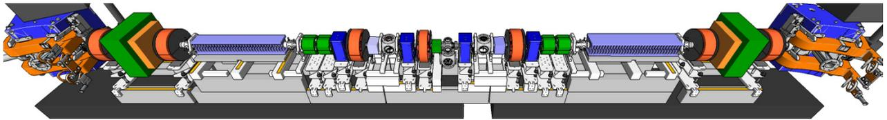
Figure 2: Integrated model of the OSC insertion in the full configuration; chicane dipoles (blue), OSC quads (small green), coupling quad (small green at center), sextupoles (orange), correctors and OSC undulators (light blue).
