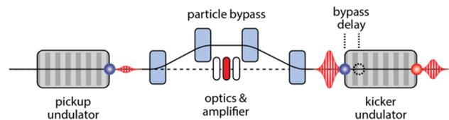
Figure 1: Simplified conceptual schematic of a transit-time OSC insertion.
