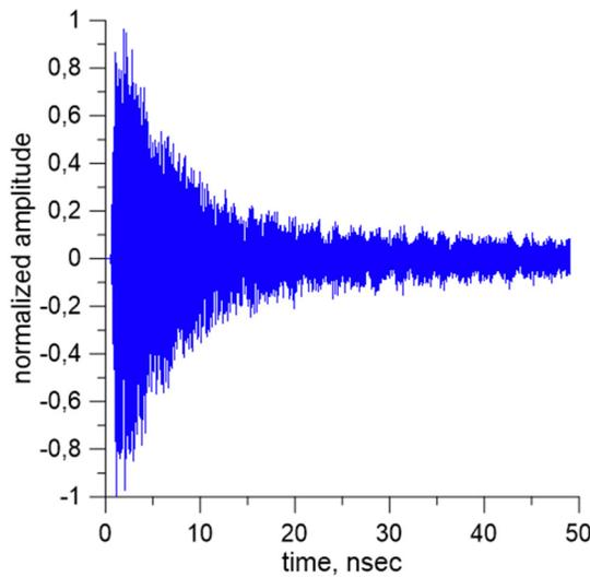
Figure 9: RF power in output of the extractor produced by single bunch.
