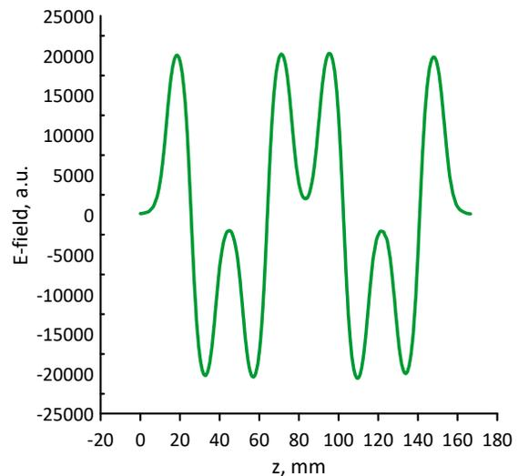
Figure 7: Accelerating field at axis of the extractor.
