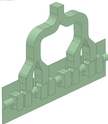
Figure 5: 11.7 GHz power extractor (a half of geometry).
