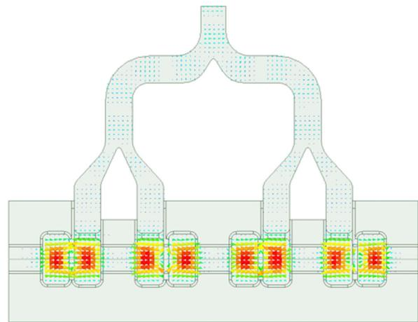
Figure 6: E-field distribution of operating mode.
