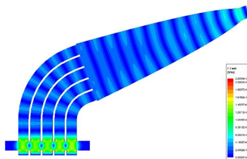
Figure 3: E-field distribution of the operating mode.
