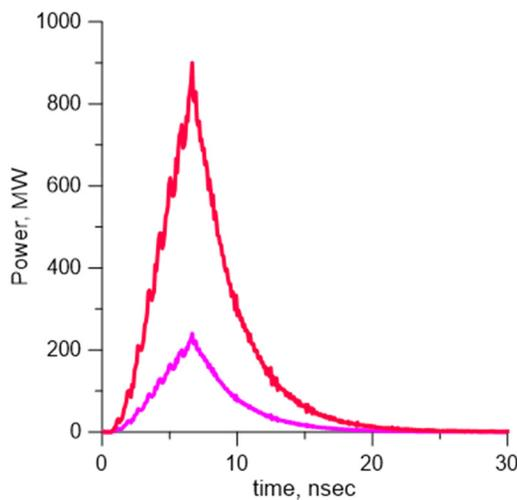
Figure 10: RF power envelope produced by eight 25 nC bunches (purple curve) and by eight 50 nC bunches (red curve).
