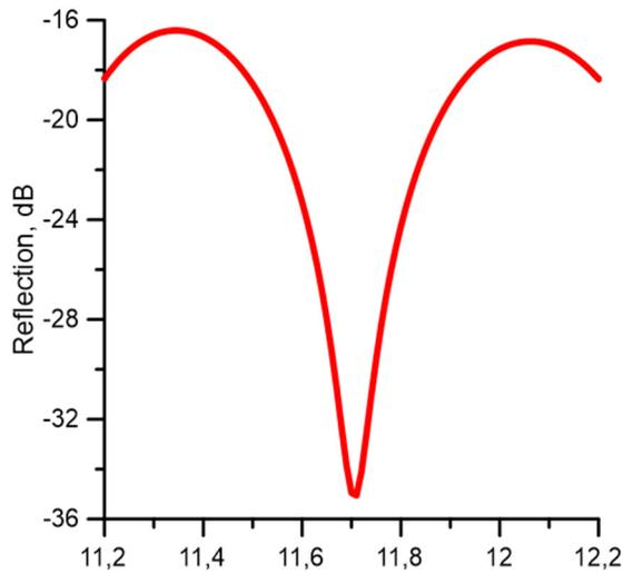
Figure 4:  $S_{11}$  parameter vs frequency.
