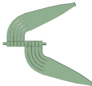
Figure 1: 5-cell side coupled accelerating structure.
