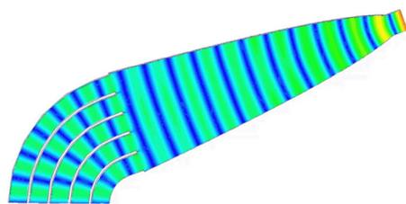
Figure 2: Instant E-field structure in feeding antenna.
