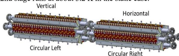
Figure 1: Dual SCAPE concept. Flux from each device can be selected by a monochromator with the energy shifts by the current bumps.
