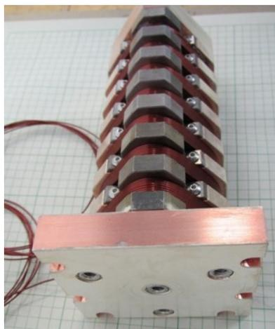
Figure 3: Prototype SCAPE magnet showing NbTi wires wound layer-by-layer. Ferromagnetic pole pieces and oxygen-free copper former are also visible.
