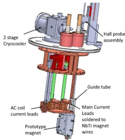
Figure 2: AC loss measurement setup.
