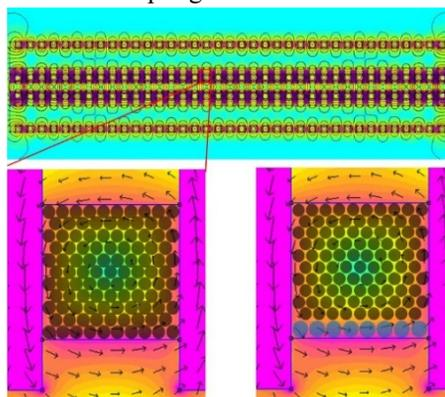
Figure 4: Top is the 2D field simulation model. Below are a single-coil pack (left) and a two-coil pack (right)—one for the AC field modulation (blue) and the other for the DC field.
