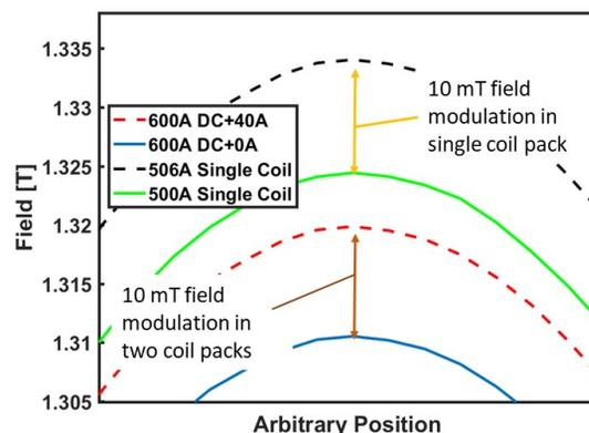
Figure 5: Field modulation for both magnets wound with single and two coil packs. The modulation is about 10 mT.
