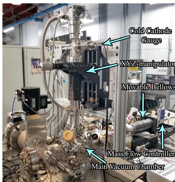
Figure 2: Gas Sheet Profile Monitor Test Stand.
