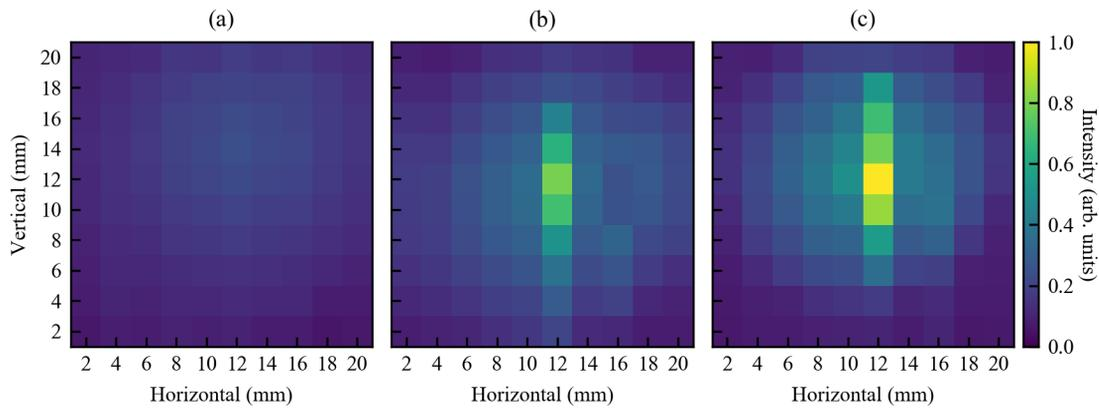
Figure 4: Slices of the transverse plane at distances of 14.68 mm (a), 9.60 mm (b) and 4.52 mm (c) from the skimmer. The skimmer–nozzle distance was 31.75 mm.
