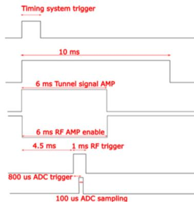
Figure 5: Timing and triggers.
