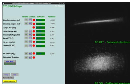
Figure 7: Screenshot of the BSM control screen with sample measurements.
