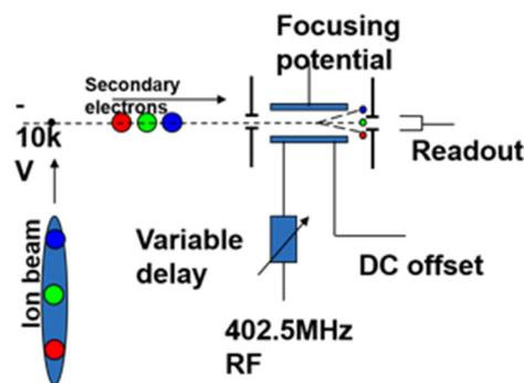
Figure 1: BSM working principle.
