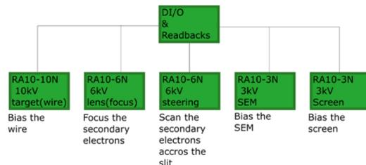
Figure 4: High voltage block diagram.
