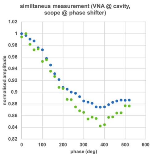
Figure 6: RF amplitude dependence on RF phase.
