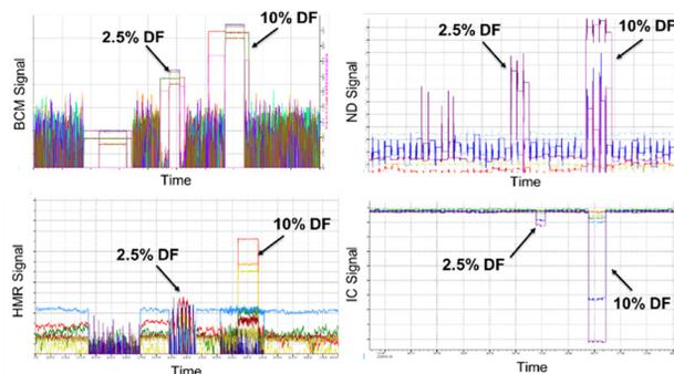
Figure 1: Concurrent detection of beam loss on BCMs, HMRs, NDs, and ICs for tests with DF of 2.5% and 10%.
