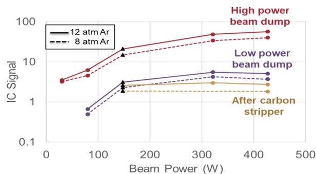
Figure 2: Ion chamber signal as a function of beam power. Beam was directed to the high-power beam dump.
