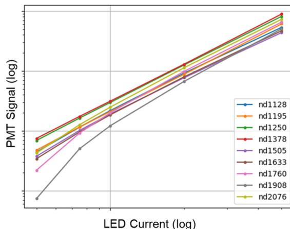
Figure 4: Neutron detector signal at a bias of -700 V, as a function of test LED current. Two detectors show non-linearity for small LED light output (current  $<1 \mu$ A).
