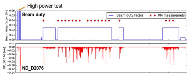
Figure 3: Neutron detector signal spikes corresponding to usage of an adjacent profile monitor (dots).
