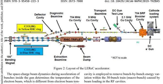
Figure 2: Layout of the LEReC accelerator.
