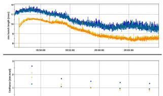
Figure 4: 6-D cooling of a 111x111 bunch RHIC store at 3.85 GeV (1.6 MeV electrons, 15mA 9 MHz CW current). Top plot - reduction of bunch length. Bottom plot - reduction of transverse beam emittances (two rings, two planes).
