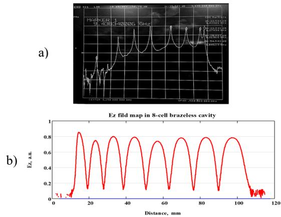
Figure 5: 8-cell brazeless cavity tuning results: a) resonance frequency spectrum; b) accelerating field bead pull measurement.
