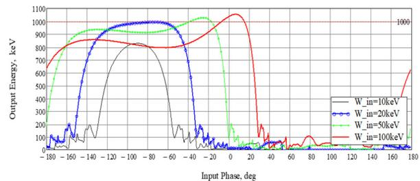
Figure 3: Energy gain vs initial accelerating field phase and input beam energy.
