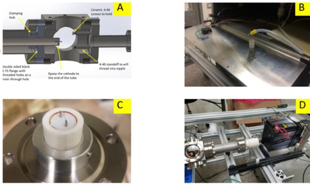
Figure 6: DC gun engineering. A) Overall layout. B) Modulator high voltage feedthrough. C) Gun packaging. D) DC gun stand assembly with floating battery for filament heating (safety cage removed).
