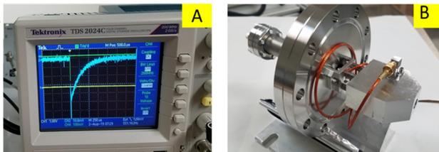
Figure 7: Accelerated beam signal on beam halo monitor: A) low beam current ( $< 50\mu\text{A}$  pulse,  $10^{-5}$  duty factor) signal; B) beam halo monitor with silicon sensor inside.
