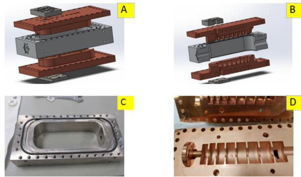
Figure 4: Brazeless split block engineering. A) Brazeless split block – knife loaded stainless-steel middle is being pressed by two copper halves. B) Brazeless split block – cut away view. C) Stainless-Steel block fabricated. D) Two copper RF halves.
