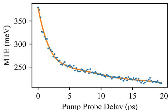
Figure 3: MTE of the pump probe photoemitted electrons as pump probe delay is changed. A smoothed curve, orange, is included to help guide the eye.
