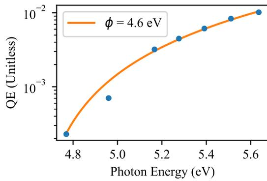
Figure 1: Quantum efficiency (QE) as a function of photon energy for the GaAs (110) sample. Photocurrent was measured at five intensities for each photon energy to accurately determine the QE and to ensure there was no multiphoton photoemission. A quadratic model, shown in orange, was fit to the data with workfunction ( $\phi$ ) as a fit parameter. The fit value of the workfunction was  $\phi = 4.6$  eV.
