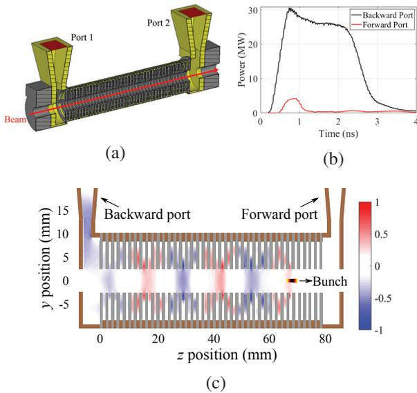
Figure 3: Numerical simulations in the CST Particle Studio. (a) Complete model of the 40-cell Stage-I structure. (b) Extracted microwave power at the two output ports. (c) Plot of longitudinal electric field  $E_z$  excited by a bunch traveling to the right on the middle plane.
