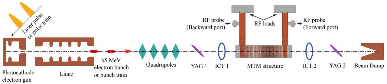
Figure 1: Schematic diagram of the experimental facilities at AWA.
