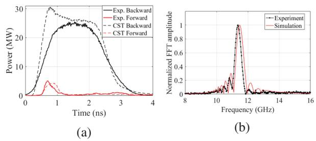
Figure 4: Measured RF pulse from a single 45 nC bunch in the Stage-I experiment benchmarked with the CST PIC simulation. (a) Microwave power in the two ports. (b) Frequency spectrum of the signal at the backward port.
