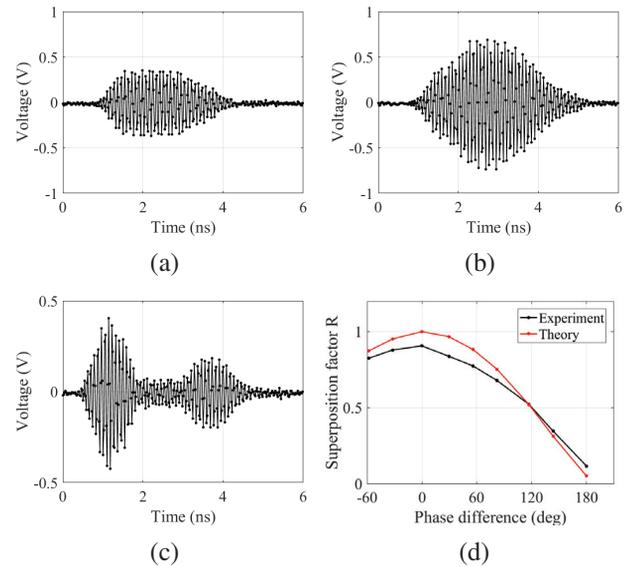
Figure 5: Beam test results from two 4 nC bunches. Voltage signal from (a) a single bunch, (b) two bunches with 0 degree phase difference, (c) two bunches with 180 degrees of phase difference of X-band. (d) Variation of the superposition factor  $R$  with the phase difference in X-band between the two bunches.
