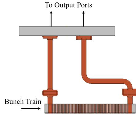
Figure 7: Drawing of the 100-cell Stage-II MTM structure. One straight waveguide and one bent waveguide are brazed onto the top flange of the vacuum chamber, and the longer 20 cm long structure is suspended by the two waveguides.
