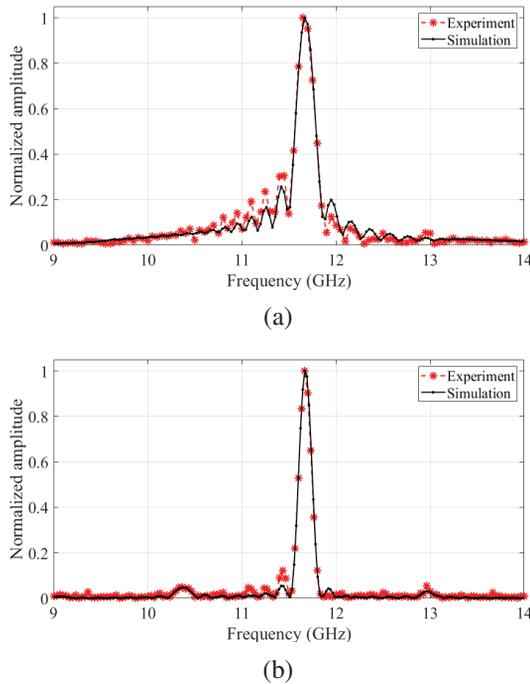
Figure 9: Frequency spectra of the Stage-II structure driven by: (a) a single bunch, (b) a train of 8 bunches.
