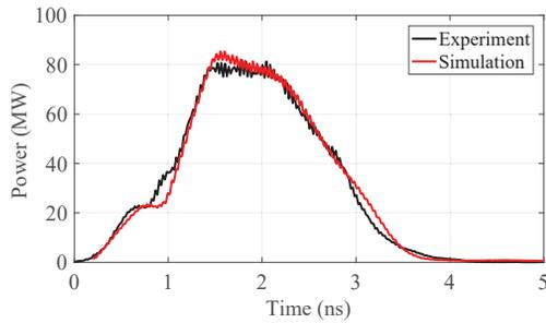
Figure 6: Highest microwave power in the Stage-I experiment from two bunches with a total charge of 85 nC in phase with each other.
