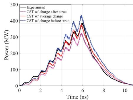
Figure 8: Highest microwave power from 8 bunches with a total charge of 224 nC before the structure and 194 nC after the structure (beam transmission 86.5%). The three simulation curves are plotted assuming that the effective charge contributing to the extracted RF power is the charge before the structure, the charge after the structure and the average of the two.
