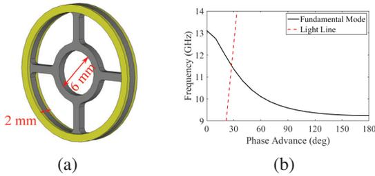
Figure 2: MTM unit cell design. (a) Unit cell geometry. Beam aperture is 6 mm. The yellow part is in copper and the grey part is in stainless steel. (b) Dispersion curve (frequency vs. phase advance per unit cell) of the fundamental TM mode showing an interaction frequency of 11.42 GHz.
