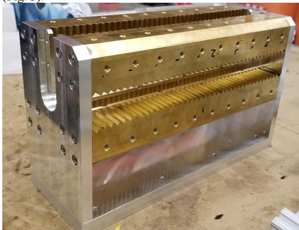
Figure 5: Prebuncher strongback assembly.
