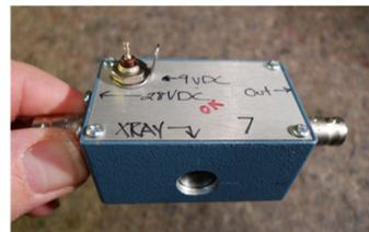
Figure 2: Packaging of the full detector. The hole on the front was aligned with the collimator in the shielding and covered with opaque tape so that light would not trigger the detector.
