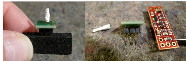
Figure 1: Scintillator mounted on SiPM detector (left), LYSO scintillator, SiPM detector and preamplifier.
