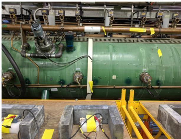
Figure 3: Detector placement for first test. The brick on the front has a 1 cm hole to act as a collimator and limit the detector's field to only one gap of the cavity. This three-brick housing proved ineffective in shielding the detectors from X-rays being produced in adjacent gaps.
