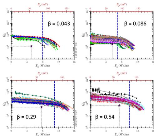
Figure 3: RF measurements on FRIB cavities at 2 K, showing high-field  $Q$ -slope above  $B_p \sim 85$  mT.
