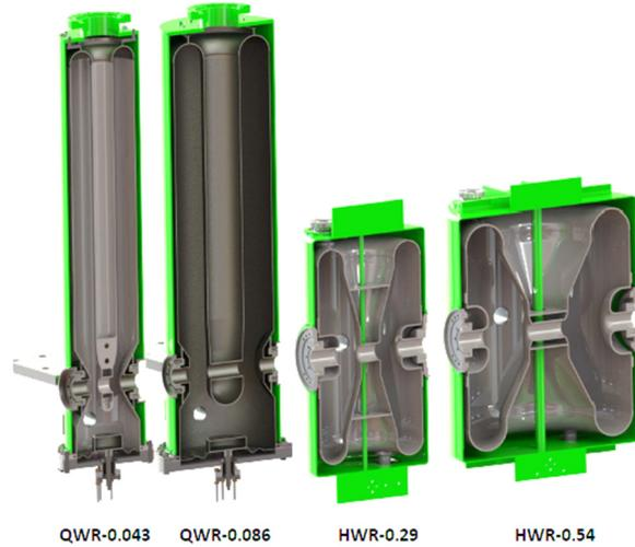
Figure 1: Isometric sectional views of jacketed cavities.
