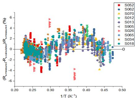
Figure 4: Relative difference between measured  $R_s$  and fitted  $R_s$  as a function of  $1/T$  for ten  $\beta = 0.29$  HWRs.
