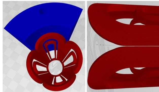
Figure 4: Coil and yoke model for iQDS1a 3D analysis.
