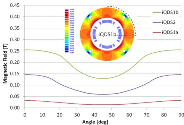
Figure 3: Fringe field at reference gradient in the downstream ion quadrupoles (field is plotted along dotted line).
