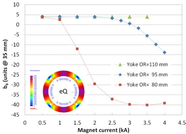
Figure 2: Saturation effect on  $b_6$  in the electron quadrupole as a function of current and the yoke outer radius.
