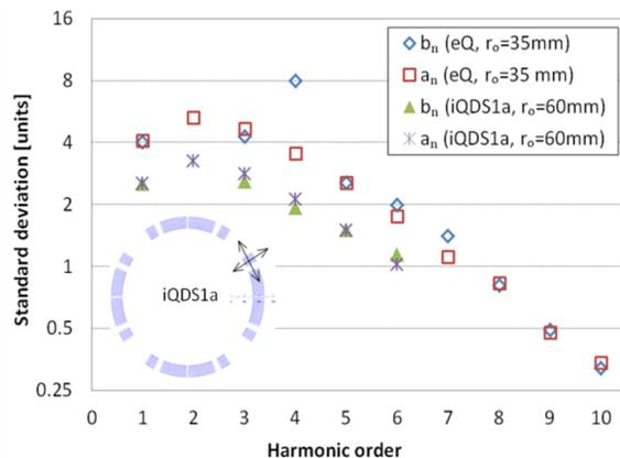
Figure 1: Random errors for conductor block positioning tolerances of  $\pm 100 \mu\text{m}$  in radial and azimuthal direction.
