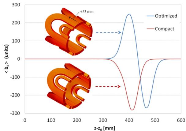
Figure 5: Comparison of  $b_6$  as a function of  $z$  in iQDS1a for the compact vs. field quality optimized end geometry.
