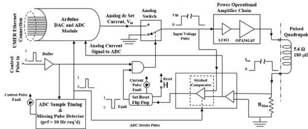
Figure 1: Block diagram of entire amplifier module.
