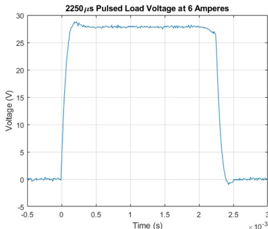
Figure 5: Pulsed load output voltage.
