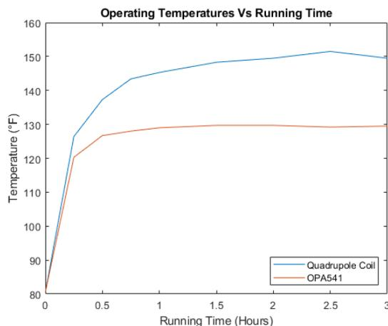
Figure 6: Operating temperatures of injection quadrupole coil and OPA541.
