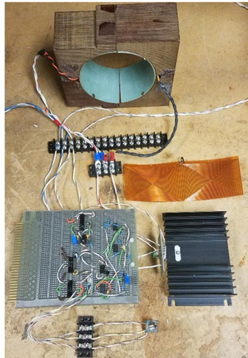
Figure 3: Picture of full circuit prototype. (Clockwise from top) injection quadrupole, mylar coated magnet coil, OPA541, reset switch, amplifier and safety circuitry.
