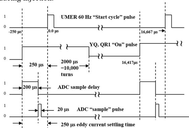
Figure 2: Timing diagram for the pulsed quadrupole amplifier.
