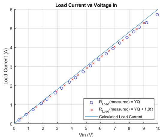
Figure 4: Measured and Calculated Load Current.
